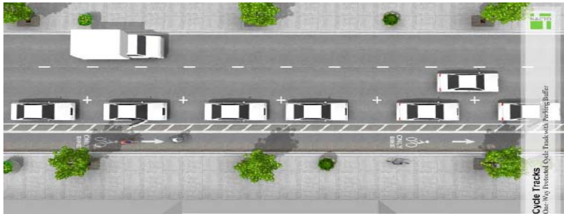
One-way cycle track with on-street parking as the buffer from the motor vehicle travel lanes. Note the use of “parking T’s” to designate the on-street parking spaces. (Source: NACTO Urban Bikeway Design Guide)
