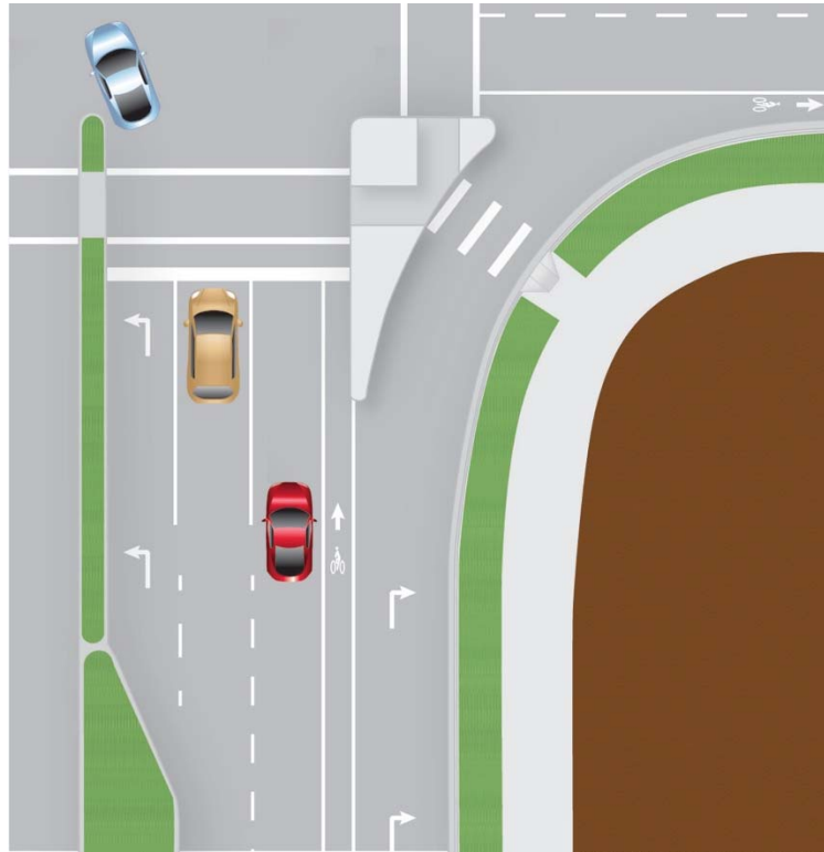
Traffic channelization is an effective mitigation strategy when intersection radii reduction is not an option. (Credit: Michele Weisbart)
