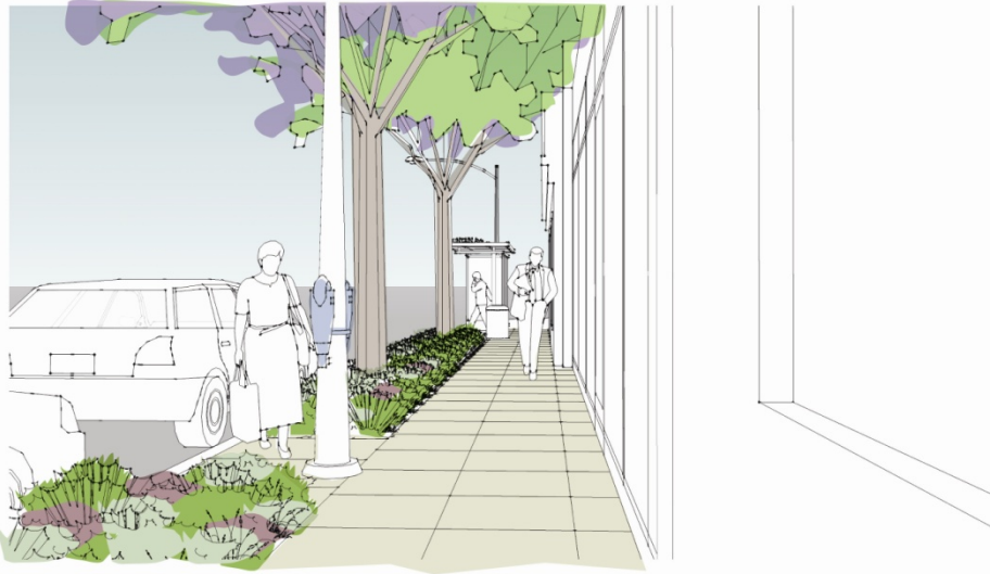
Walking path across understory landscaping provides access from parked cars to sidewalk (Credit: Patricia Smith)
