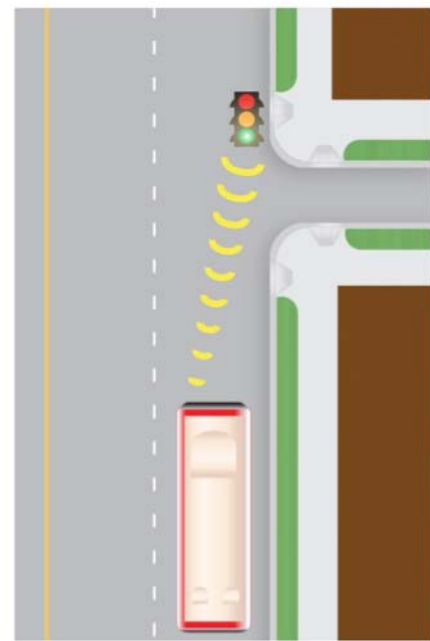
Signal-priority technology can help to reduce delay for buses (Credit: Michele Weisbart)
