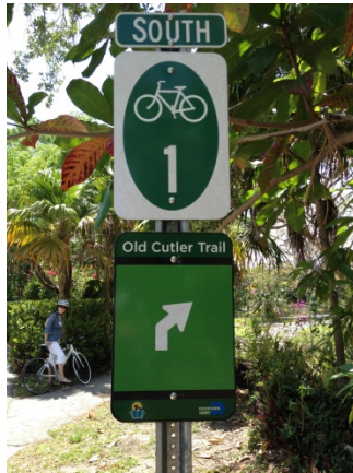
Numbered bicycle route signage at a turn location. Note that if the arrow turn plaque were removed, this would be a confirmation sign.
