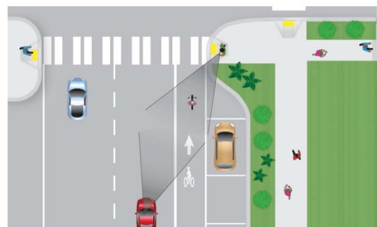
Curb extensions (Credit: Michele Weisbart)
