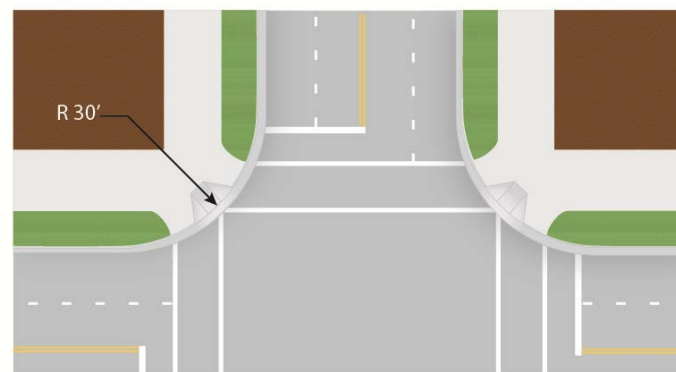
Tighter corner radii reduce crossing distance and slow turning traffic. (Credit: Michele Weisbart)
