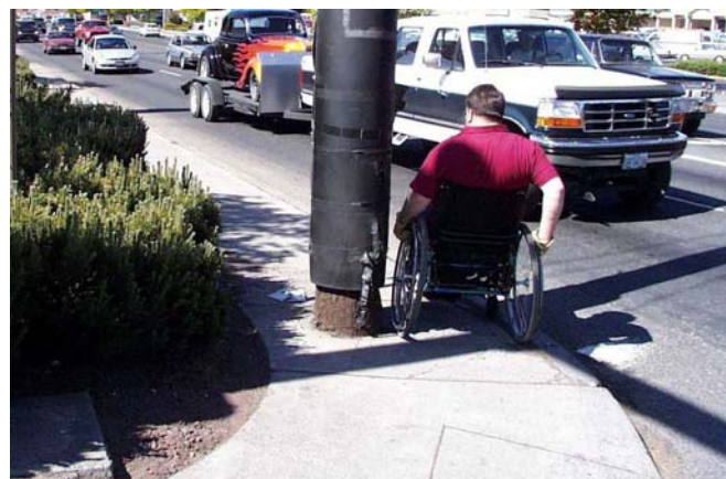
Obstructions can make passage difficult or impossible for wheelchair users. (Credit: Michael Ronkin)
