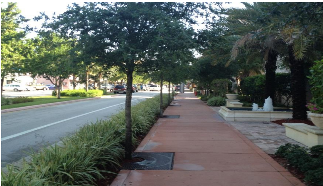
Landscaped buffer between pedestrians and motor vehicles (Credit: Kimley-Horn and Associates, Inc.)
